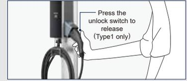
2. Releasing the hooked cable to expand to connect the EV connector inputs.
